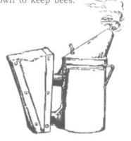
Bottom of smoker gets hot enough to ignite dry grass and leaves. Beekeepers often work in dry grass and leaves. While tin smoker body expands when hot, Niconel "memory metal" top shrinks when heated to make opening and re-fueling nearly impossible.
